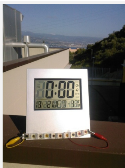
Fig. 2. Digital clock powered by natural dye solar cells
